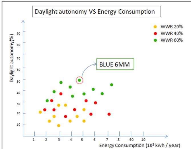
FIG. 15: Daylight autonomy and energy consumption.
