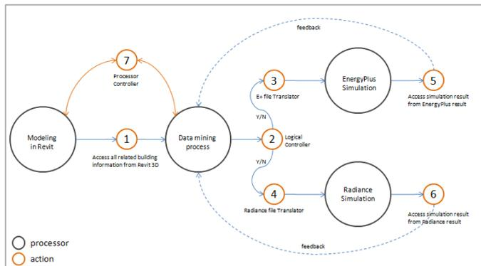
FIG. 9: Overview of proposed data-driven workflow
