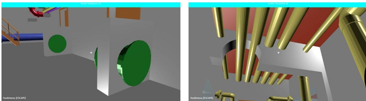
Figure 3: Discoveries in the water production plants case: an unconnected pipe section (left) and a potential error in the number of pipes (right)
