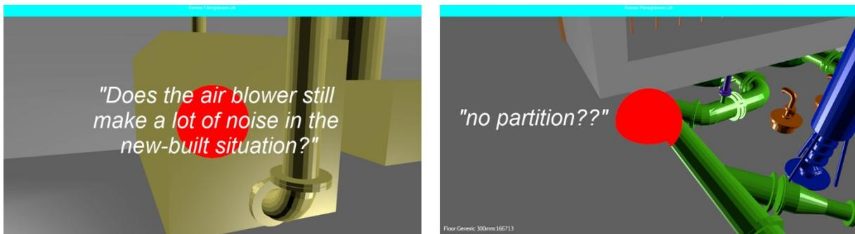
Figure 5: Examples of feedback on a design proposal in the water production plants case (text pasted on original screenshots): a comment about the noise level produced by a number of air blowers (left) and a comment about the absence of partitions to protect from falling down (right)
