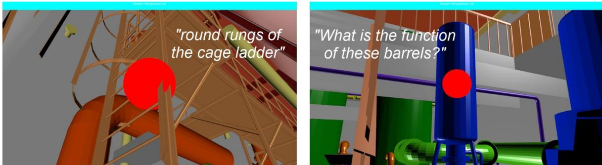
Figure 4: Examples of feedback on a design proposal (text pasted on original screenshots). Clients participate in design discussions about issues they previously identified in the virtual environment: the ergonomics of holding a specific type of rungs of a cage ladder (left) and the function of some “barrels” in the basement of the proposed design (right)
