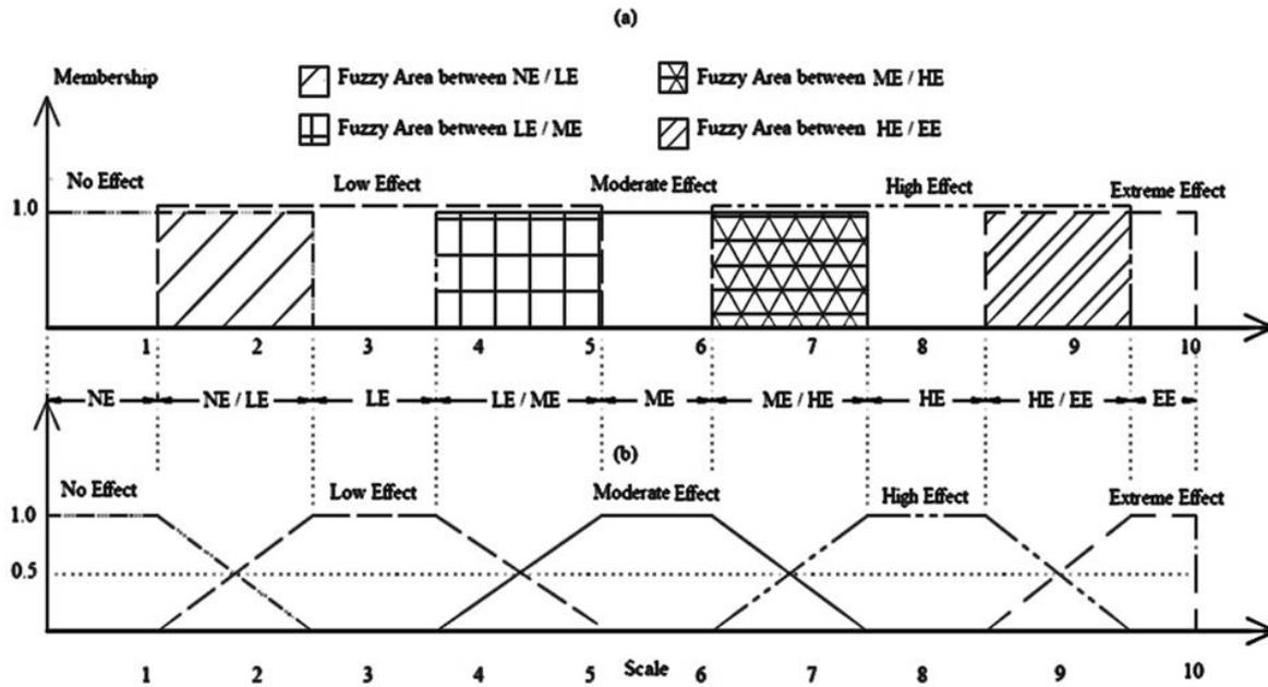
Figure 5: Fuzzy linguistic - numeric conversion scheme: preliminary (a) and final (b)
