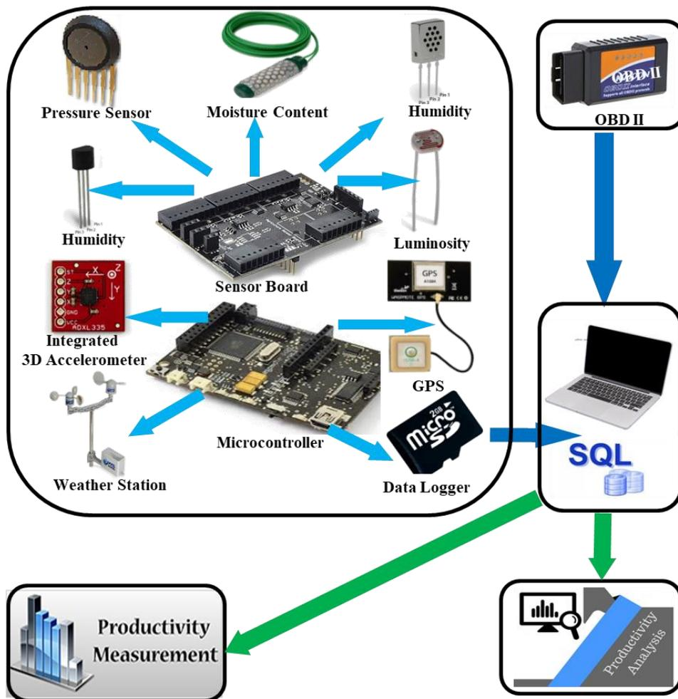
Figure 13: The Architecture of the Proposed Customized Data Acquisition System
