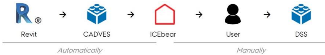
Figure 14. Data transfer principle between Revit, ICEbear and the plug-in
