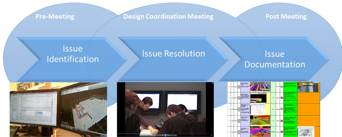
FIG. 5: Three critical steps in the BIM-based design coordination process. Design coordination issue identification, resolution, and issue documentation.
