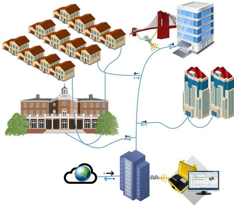
FIG. 1: Schematic demonstration of using existing urban fibre optic infrastructure for transmitting sensor data in structural monitoring.
