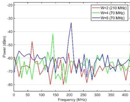
FIG. 7: The RF signal power received for distance of 20 km for all nodes.
