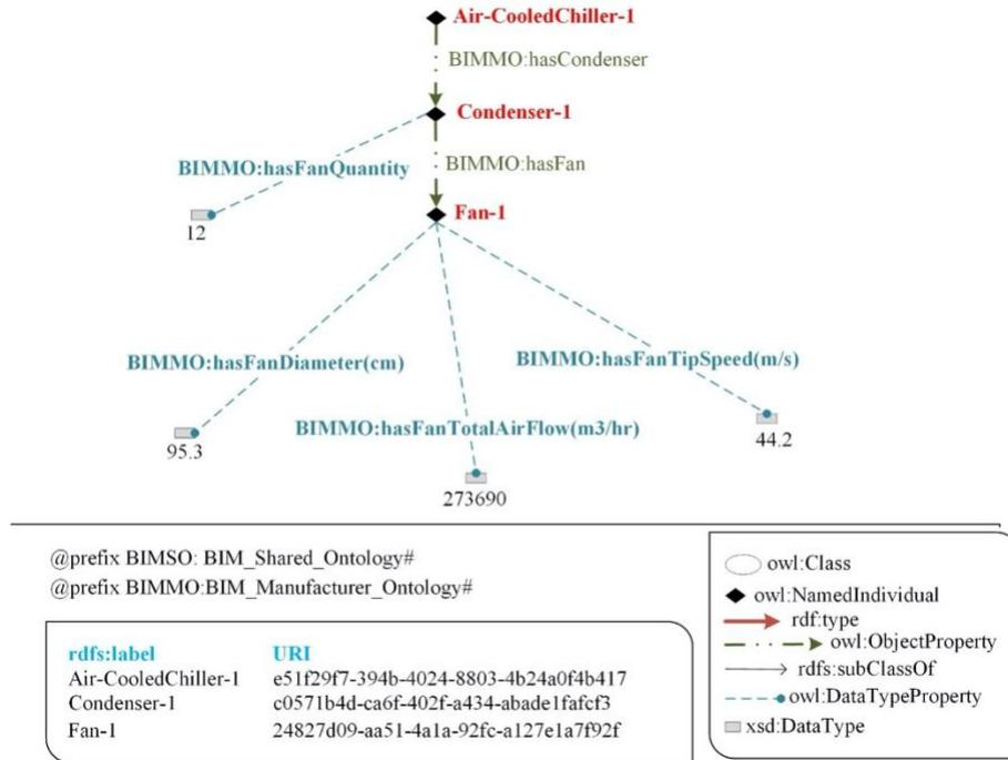
FIG. 14: A chiller's condenser properties
