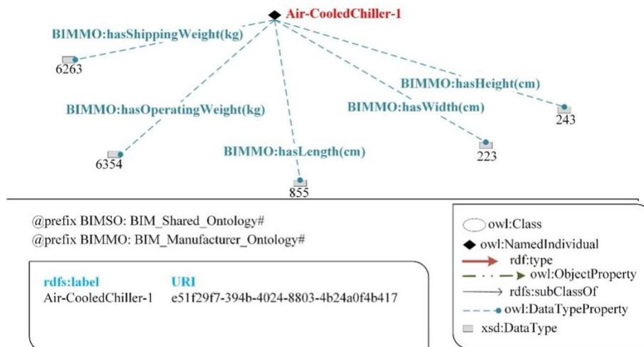
FIG. 15: A chiller's weight and dimensions
