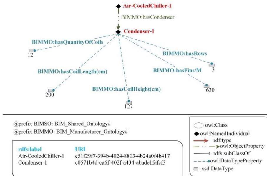
FIG. 13: A chiller's condenser properties
