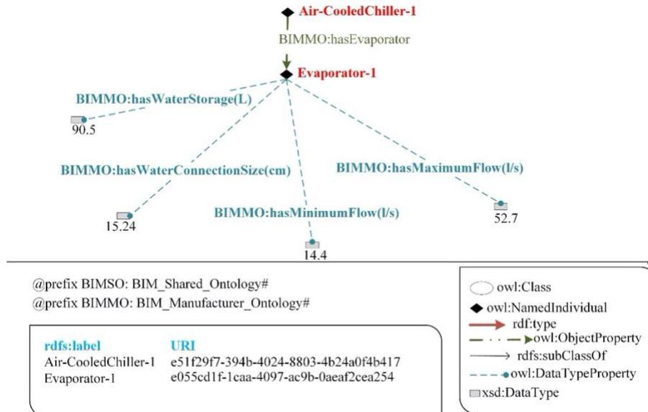
FIG. 12: A chiller's evaporators properties
