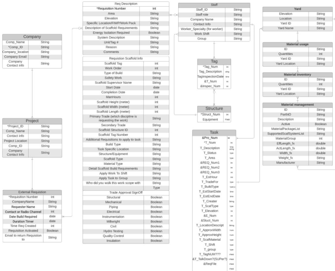
FIG. 5: Sample proposed entity relationship diagram of scaffolding management system.
