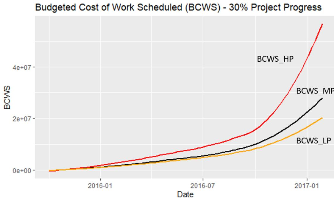
FIG. 7: Budgeted cost of work scheduled (BCWS) based on 30% project progress.
