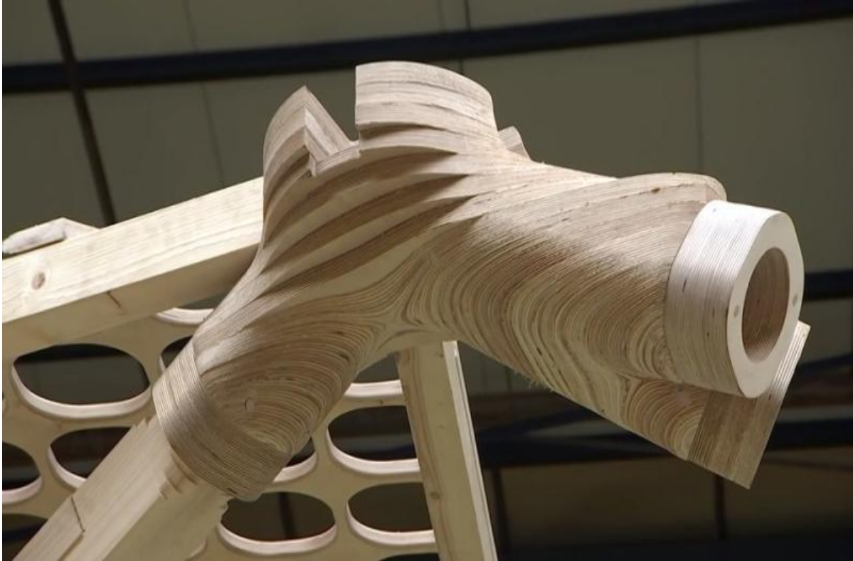
Figure 9: Connection or assembly by Stratoconception® for timber construction.
