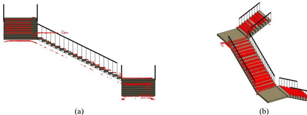
Figure 9: Fitting parametric staircase model to points; (a) Vertical alignment of the parametric model toward the staircase points (term  $G$ ), (b) placement of the parametric model planes on the staircase points (term  $F$ ).
