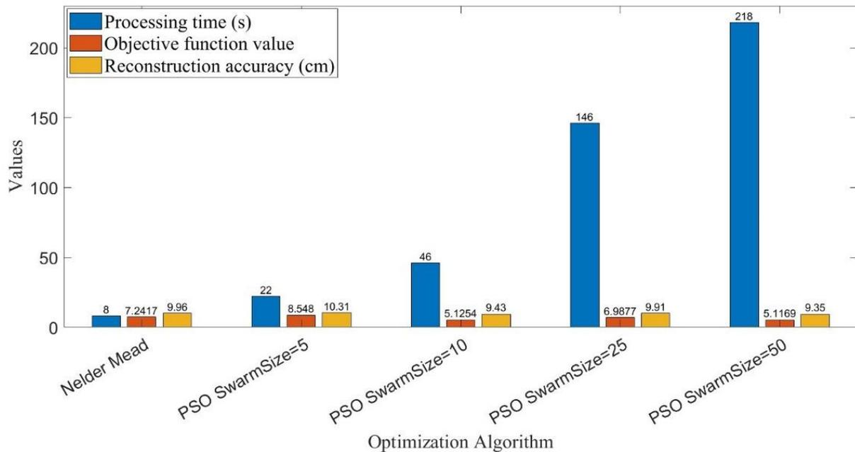
Figure 19: Evaluating the impact of the selected optimization algorithm on model fitting step: a quantitative comparison of overall objective function values, reconstruction accuracy, and the processing time required to fit the digital staircase model.
