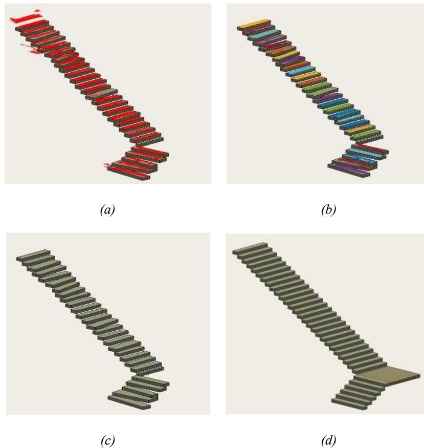
Figure 20: The results of creating a digital staircase model for TUM Floor 4 data using the data-driven approach and the proposed parametric modeling approach include: (a) separated staircase points, (b) separation of stair tread planes using the data-driven method, (c) creation of the digital staircase model using the bounding box fitting algorithm, and (d) creation of the digital staircase model using the proposed parametric modeling method.
