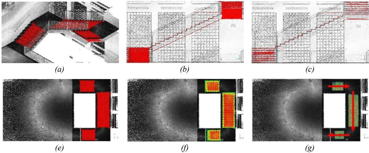
Figure 3: Interpretation of staircase configuration: (a) extracted staircase points, (b) the staircase points projected on Y-Z plan, (c) grid-based noise filtering and removing the uncommon inclined planes beneath the stair steps, (d) the staircase points projected on X-Y plan, (e) 3D point density feature calculation, (f) the detected stair flows.
