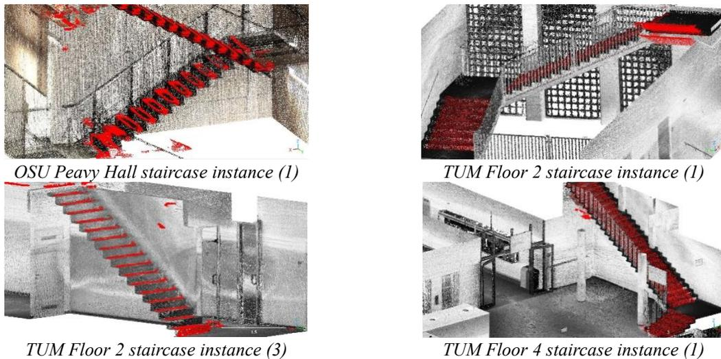
Figure 10: The results of the staircase points separation on the test data using the proposed method (rectangular configuration).
