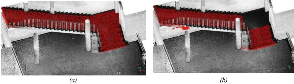
Figure 12: The result of staircase point separation for TUM Floor 4 data: (a) the ground truth for staircase points separation, (b) the result of staircase points separation using the proposed method.
