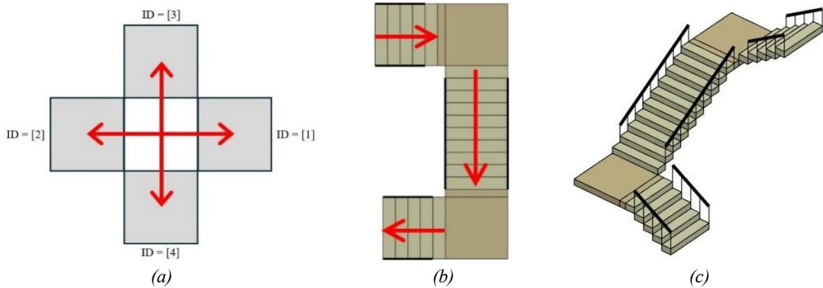
Figure 4: Determining the type of staircase based on the number of stair flows and the number of landing treads: (a) possible rotation orientations, (b) the configuration of the parametric model for the staircase instance with two landing treads and three stair flows with ID array of [1 4 2], and (c) design of the parameterized digital staircase model.
