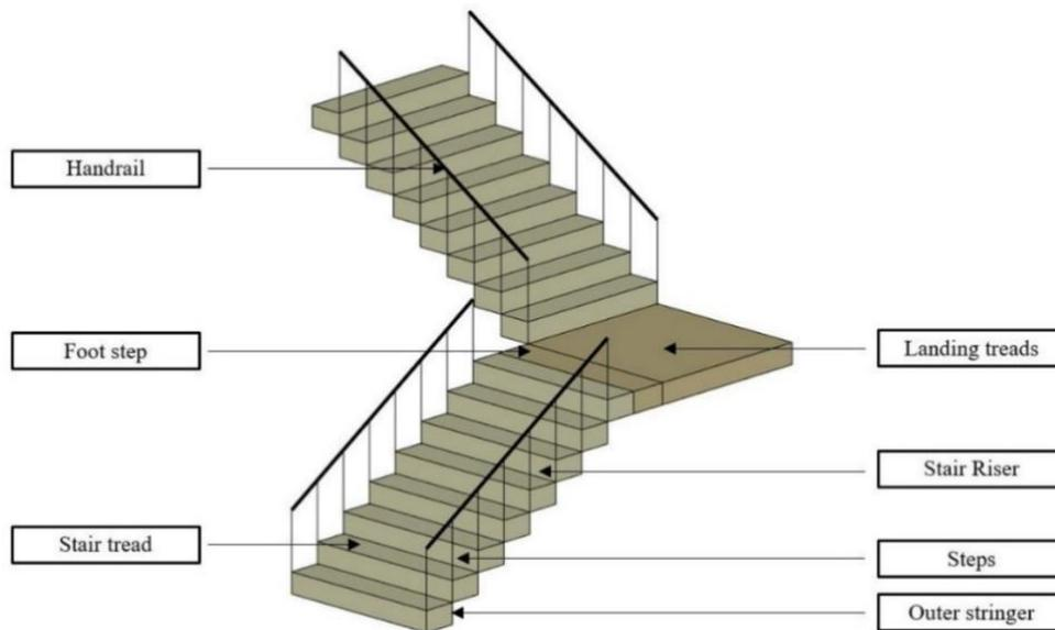
Figure 6: The components of a staircase with one Landing tread.
