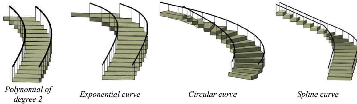
Figure 7: Representation of a non-rectangular staircase structures using various mathematical methods and equations.
