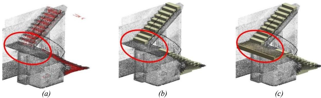
Figure 14: The effect of the maximum neighborhood distance parameter value on the result of digital staircase model creation for TUM Floor 2 staircase instance (2): (a) separated staircase instances, (b) the result of digital staircase model creation using the proposed method, and (c) correct placement of the landing tread elements in the reconstructed digital staircase model.
