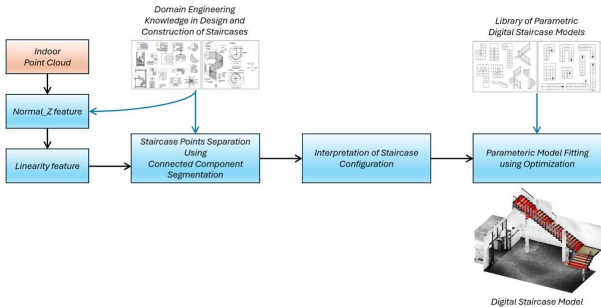
Figure 1: The proposed hybrid bottom-up, top-down workflow for creating digital staircase models using point cloud.
