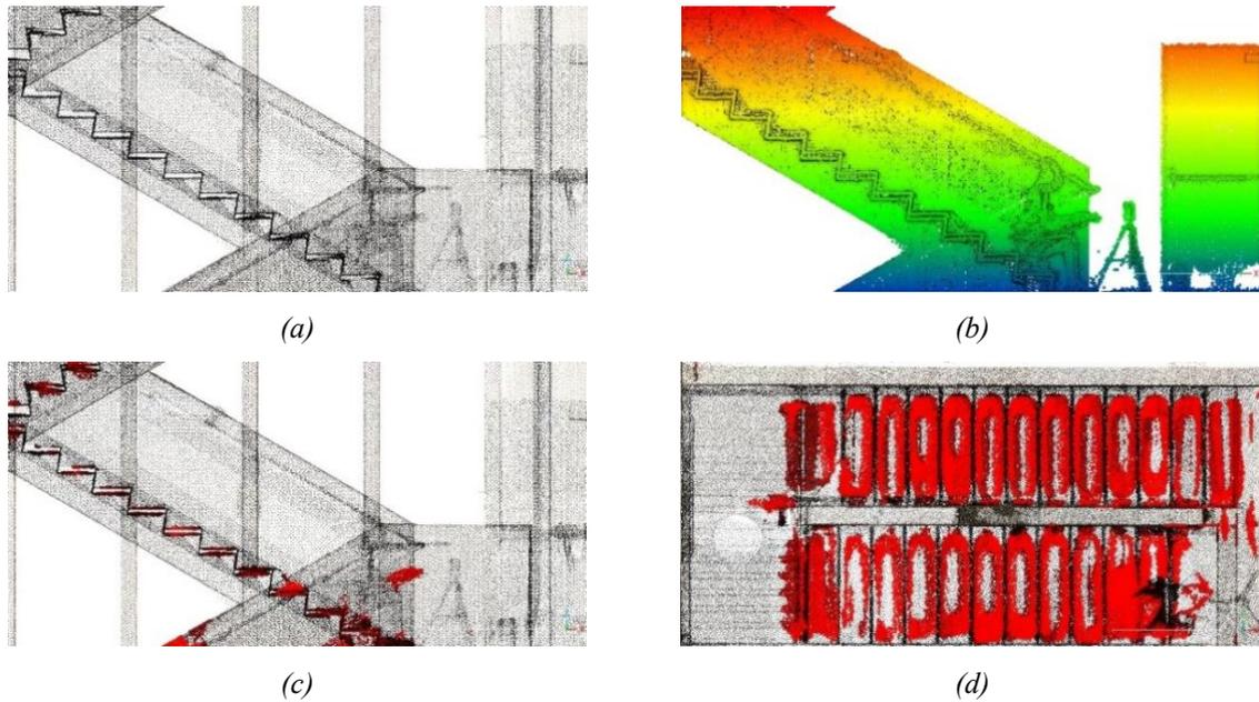
Figure 13: Error in separating staircase points in OSU Peavy Hall data: (a) the raw point cloud data, (b) the structure of the captured point cloud (including occlusions), (c) the result of the separated staircase points from side view, (d) the result of the separated staircase points from top view.
