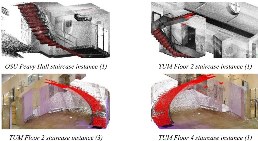
Figure 11: The results of the staircase points separation on the test data using the proposed method (non-rectangular configuration).
