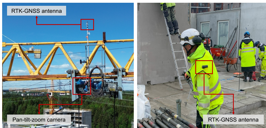
Figure 9: RTK-GNSS and camera sensors on the crane trolley (left) and embedded in workers' safety vests (right).
