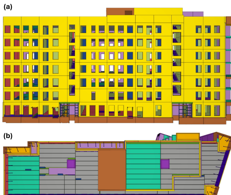
Figure 11: IFC model of the complete building structure: (a) front view and (b) top view.
