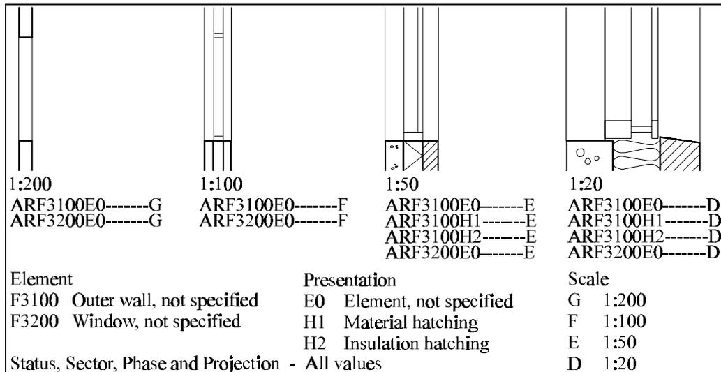
Figure 4. Detailing for different scales stored in separate layers
