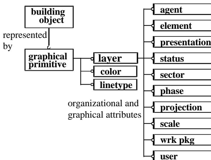
Figure 1. The way in which information is attached to graphical primitives using the proposed ISO standard
