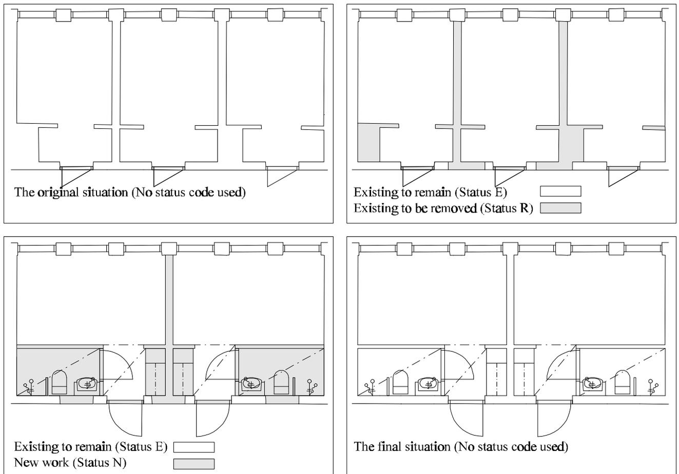
Figure 9: An example of how the status field can be used as a discriminator to produce tailor-made drawings facilitating the design and management of rebuilding.
