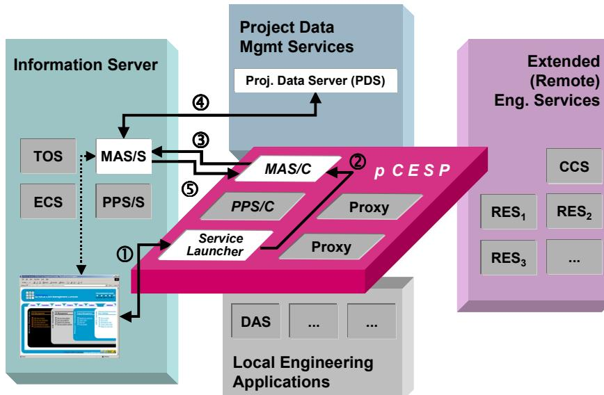
Fig. 8: Principal interoperability at business level 1 “Integration of services and project data” for the case of directly accessing the project data repositories with the help of MAS/C.
