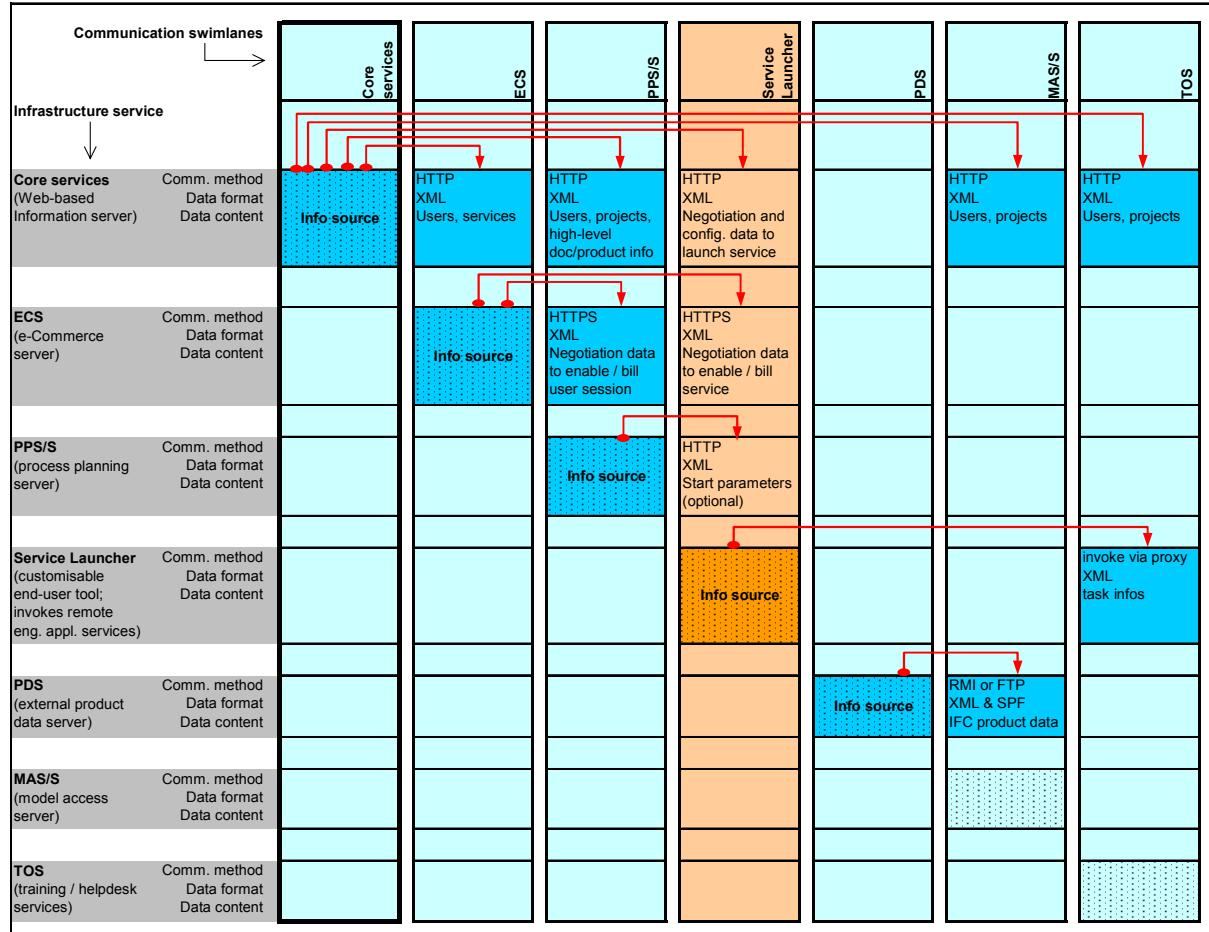
Fig.11: Interaction matrix for the CESP infrastructure services. Arrows denote the principal information flows.
