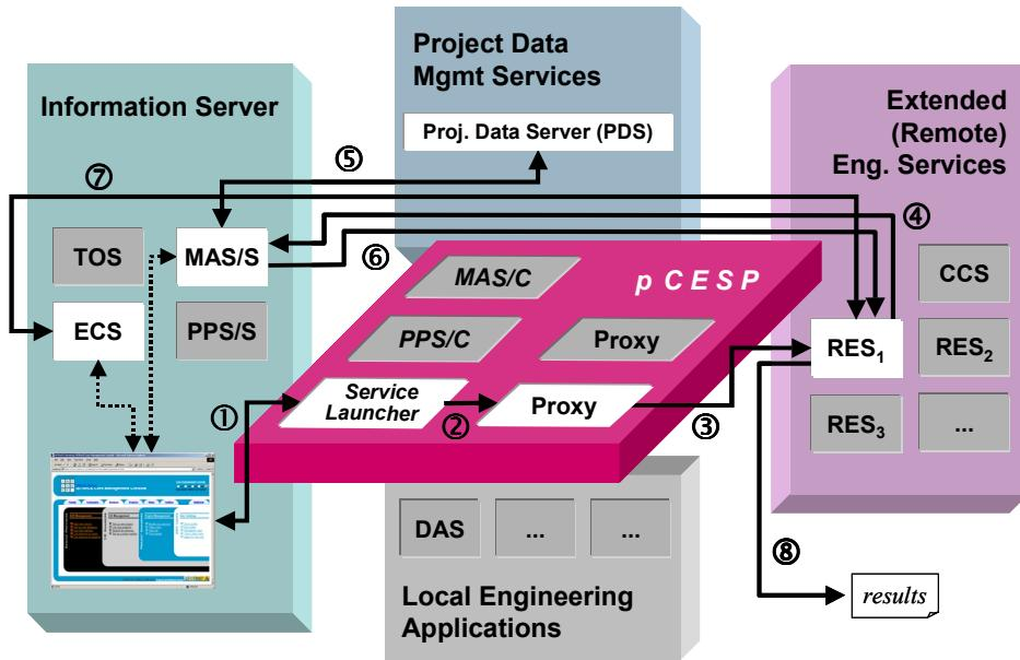
Fig. 9: Principal interoperability at business level 1 “Integration of services and project data” for the case of accessing the project data repositories by a remote engineering service.
