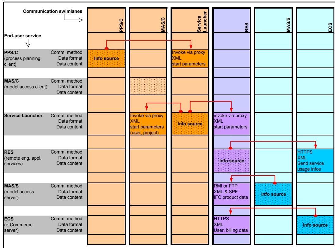
*Fig. 12: Interaction matrix showing the invocation and the principal information flows for the remote (rental) engineering services.*
